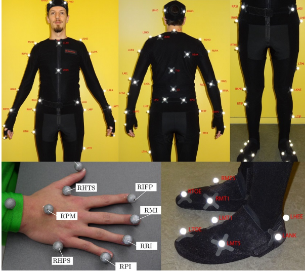
Fig. 5: MMM provides a reference marker set to be used with marker-based human capture systems.
